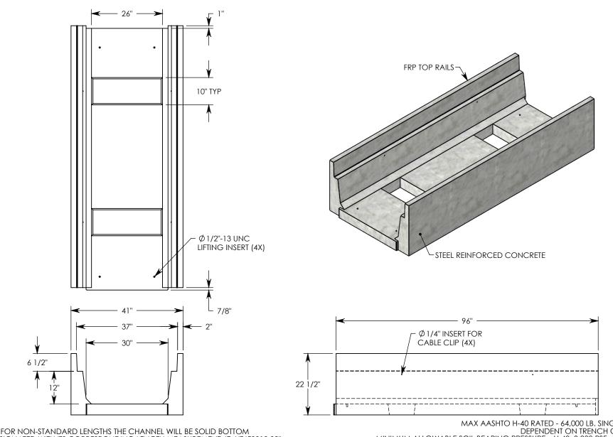
**NOTE 1:** FOR NON-STANDARD LENGTHS THE CHANNEL WILL BE SOLID BOTTOM AND DESIGNATED WITH ITS CORRESPONDING LENGTH MEASUREMENT. IE: HT6F3012 32"
