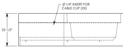
MAX AASHTO H-40 RATED - 64,000 LB. SINGLE AXLE LOAD DEPENDENT ON TRENCH COVER RATING MINIMUM ALLOWABLE SOIL BEARING PRESSURE – H-40: 3,000 PSF; H-20: 3,000 PSF
