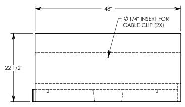
**NOTE 1:** FOR NON-STANDARD LENGTHS THE CHANNEL WILL BE SOLID BOTTOM AND DESIGNATED WITH ITS CORRESPONDING LENGTH MEASUREMENT. IE: HT6F3012 32"
