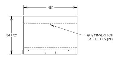
**NOTE 1:** FOR NON-STANDARD LENGTHS THE CHANNEL WILL BE SOLID BOTTOM AND DESIGNATED WITH ITS CORRESPONDING LENGTH MEASUREMENT. IE: HT6F5024 36"
