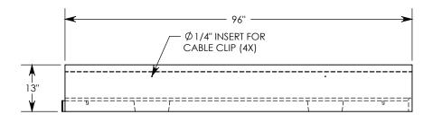
**NOTE 1:** ALL NON-STANDARD LENGTHS OF CHANNEL WILL BE SOLID BOTTOM AND DESIGNATED WITH ITS CORRESPONDING LENGTH MEASUREMENT. IE: HTF0608 32"
