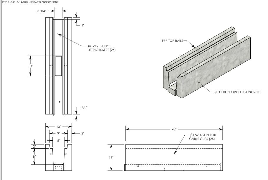
**NOTE 1:** FOR NON-STANDARD LENGTHS THE CHANNEL WILL BE SOLID BOTTOM AND DESIGNATED WITH ITS CORRESPONDING LENGTH MEASUREMENT. IE: HTF0608 32"
