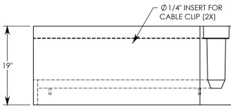
MAX AASHTO H-40 RATED - 64,000 LB. SINGLE AXLE LOAD DEPENDENT ON TRENCH COVER RATING
