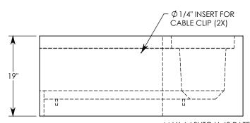
MAX AASHTO H-40 RATED - 64,000 LB. SINGLE AXLE LOAD DEPENDENT ON TRENCH COVER RATING MINIMUM ALLOWABLE SOIL BEARING PRESSURE – H-40: 5,500 PSF; H-20: 3,000 PSF
