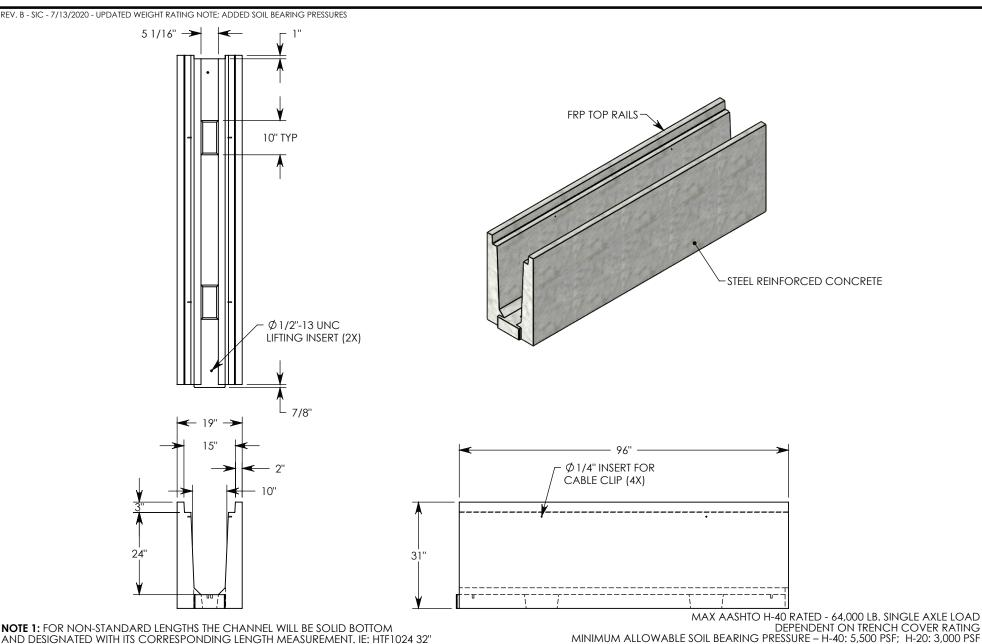
**NOTE 1:** FOR NON-STANDARD LENGTHS THE CHANNEL WILL BE SOLID BOTTOM AND DESIGNATED WITH ITS CORRESPONDING LENGTH MEASUREMENT. IE: HTF1024 32"
