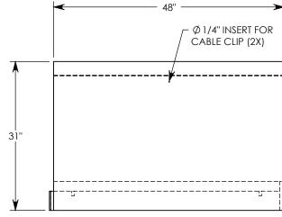
**NOTE 1:** FOR NON-STANDARD LENGTHS THE CHANNEL WILL BE SOLID BOTTOM AND DESIGNATED WITH ITS CORRESPONDING LENGTH MEASUREMENT. IE: HTF1024 32"
