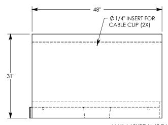
**NOTE 1:** FOR NON-STANDARD LENGTHS THE CHANNEL WILL BE SOLID BOTTOM AND DESIGNATED WITH ITS CORRESPONDING LENGTH MEASUREMENT. IE: HTF1024 32"
