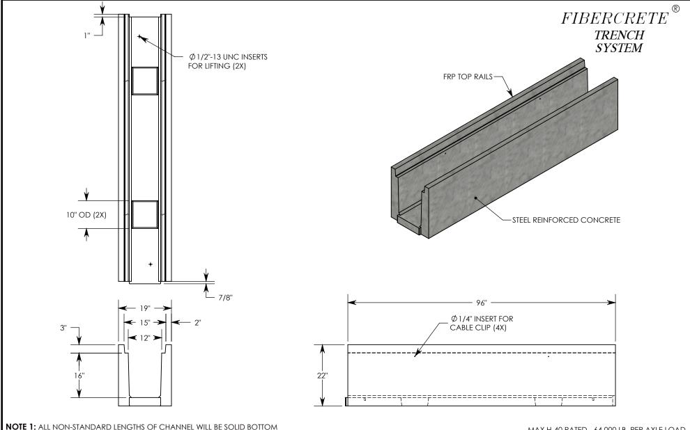
**NOTE 1:** ALL NON-STANDARD LENGTHS OF CHANNEL WILL BE SOLID BOTTOM AND DESIGNATED WITH ITS CORRESPONDING LENGTH MEASUREMENT. IE: HTF1216 32"
