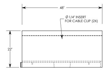
**NOTE 1:** FOR NON-STANDARD LENGTHS THE CHANNEL WILL BE SOLID BOTTOM AND DESIGNATED WITH ITS CORRESPONDING LENGTH MEASUREMENT. IE: HTF1216 32"
