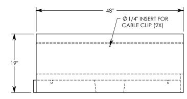
**NOTE 1:** FOR NON-STANDARD LENGTHS, THE CHANNEL WILL BE SOLID BOTTOM AND DESIGNATED WITH ITS CORRESPONDING LENGTH MEASUREMENT. IE: HTF2012 32"
