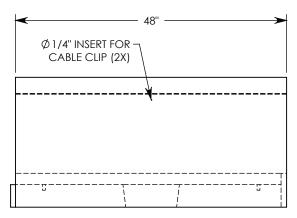
**NOTE 1:** FOR NON-STANDARD LENGTHS THE CHANNEL WILL BE SOLID BOTTOM AND DESIGNATED WITH ITS CORRESPONDING LENGTH MEASUREMENT. IE: HTF2016 32"
