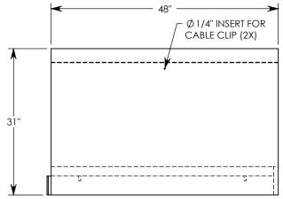
NOTE 1: FOR NON-STANDARD LENGTHS THE CHANNEL WILL BE SOLID BOTTOM AND DESIGNATED WITH ITS CORRESPONDING LENGTH MEASUREMENT. IE: HTF2024 32"
