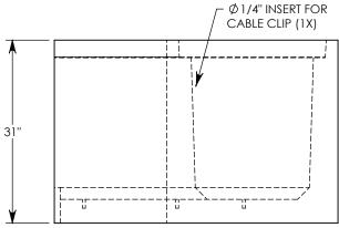
MAX AASHTO H-40 RATED - 64,000 LB. SINGLE AXLE LOAD DEPENDENT ON TRENCH COVER RATING MINIMUM ALLOWABLE SOIL BEARING PRESSURE – H-40: 4,000 PSF; H-20: 3,000 PSF
