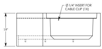
MAX AASHTO H-40 RATED - 64,000 LB. SINGLE AXLE LOAD DEPENDENT ON TRENCH COVER RATING MINIMUM ALLOWABLE SOIL BEARING PRESSURE – H-40: 3,500 PSF; H-20: 3,000 PSF
