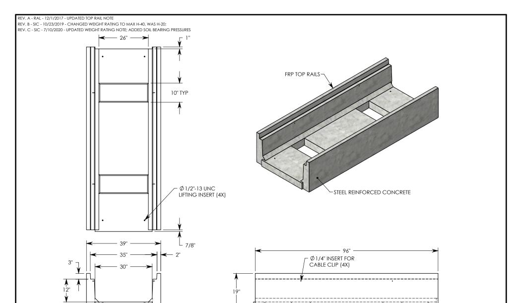
**NOTE 1:** FOR NON-STANDARD LENGTHS THE CHANNEL WILL BE SOLID BOTTOM AND DESIGNATED WITH ITS CORRESPONDING LENGTH MEASUREMENT. IE: HTF3012 32"
