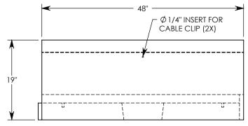
**NOTE 1:** FOR NON-STANDARD LENGTHS, THE CHANNEL WILL BE SOLID BOTTOM AND DESIGNATED WITH ITS CORRESPONDING LENGTH MEASUREMENT. IE: HTF3012 32"
