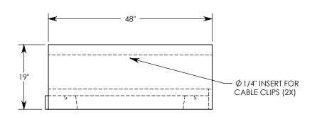
**NOTE 1:** FOR NON-STANDARD LENGTHS THE CHANNEL WILL BE SOLID BOTTOM AND DESIGNATED WITH ITS CORRESPONDING LENGTH MEASUREMENT. IE: LTF2412 36"
