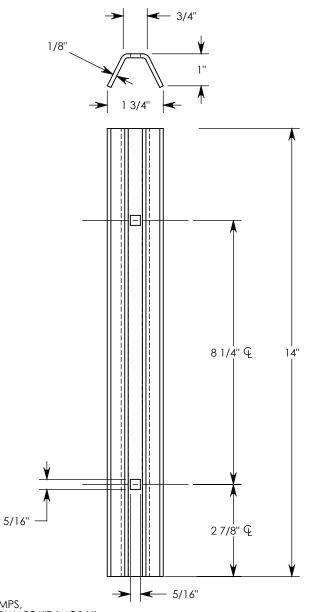
**NOTE 1:** THE MGS-SH KIT CONSISTS OF 4 OF THESE CLAMPS, WHICH ARE USED IN ADDITION TO THE STANDARD HARDWARE KIT (MGS-H)
