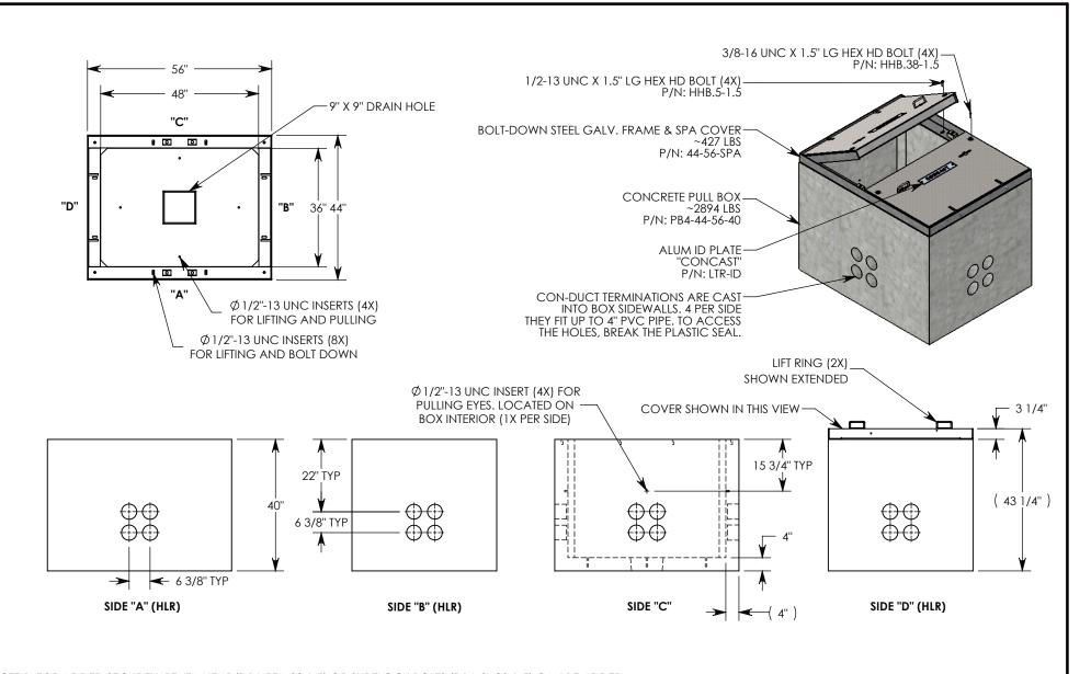
**NOTE 1:** FOR ADDED SECURITY, PENTA HEAD(P/N: PTA.38-1.5) OR SURELOCK BOLTS (P/N: SL.38-1.5) CAN BE ADDED **NOTE 2:** FOR PVC SIZES SMALLER THAN 4", USE CONCAST RC41 (REDUCING COUPLER).
