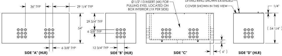
NOTE 1: FOR PVC SIZES SMALLER THAN 4", USE CONCAST RC41 (REDUCING COUPLER) NOTE 2: FOR ADDED SECURITY, PENTA HEAD BOLTS (P/N: PTA.5-1.5) CAN BE ADDED
