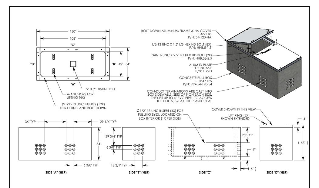
NOTE 1: FOR PVC SIZES SMALLER THAN 4", USE CONCAST RC41 (REDUCING COUPLER).
