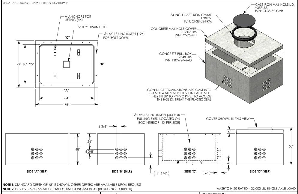
DRAWN BY: JESSE GUTTING CREATED DATE: 3/10/2020 REVISION LEVEL: A 8/2/2021 SAVED DATE: SAVED BY: jgutting WEIGHT: MATERIAL: **NOTED** 13485 LBS.
