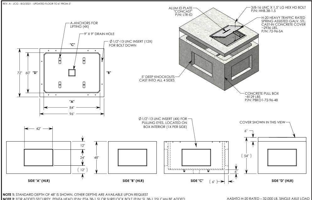
NOTE 2: FOR ADDED SECURITY, PENTA HEAD (P/N: PTA.38-1.5) OR SURELOCK BOLT (P/N: SL.38-1.25) CAN BE ADDED
