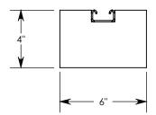
7,500 PSI CONCRETE SUPPORT BLOCK IS DESIGNED TO FIT INSIDE ANY STANDARD CONCAST 20" ID CHANNEL
