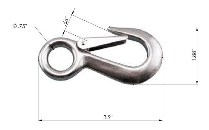
**NOTE 1:** 300 LB. WORKING LOAD LIMIT. WORKING LOADS ARE BASED ON GRADUAL PULL, NOT SHOCK LOADS.
