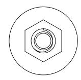
FOR USE WITH CONCAST PRODUCTS SUCH AS CURBS & FPS STYLE FLAT PADS. 70,000 PSI MINIMUM TENSILE STRENGTH. STAINLESS STEEL VERSION AVAILABLE AS CONCAST PART NUMBER WA.5-3.75-SS
