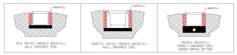
A bed of coarse rock is recommended to bring the yard up to final grade. The final grade must be maintained flush with the top of the road crossing sections. At high frequency traffic areas, the earth should be well compacted. A cement slurry or a concrete apron is also recommended. This will reduce impact loading and possible chipping and cracking on the edges of channels.
