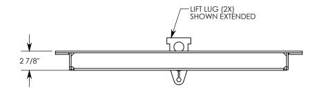
NOTE 1: FOR ADDED SECURITY, PENTA HEAD (P/N: PTA.38-1.5) OR SURELOCK BOLTS (P/N: SL.38-1.25) CAN BE ADDED NOTE 2: TREAD ON DIAMOND PLATE ADDS 1/8" TO OVERALL HEIGHT
