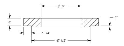
**NOTE 1:** USE OPTIONAL 4" TALL EXTENSION/GRADE RINGS TO INCREASE HEIGHT OF COVER OPENING. P/N: HE-42 **NOTE 2:** CAST IRON MANHOLE LID & FRAME ARE INCLUDED WITH THE FINAL PULL BOX ASSEMBLY.
