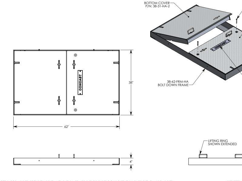
NOTE 1: FOR ADDED SECURITY, PENTA HEAD (P/N: PTA.38-2.5) OR SURELOCK BOLTS (P/N: SL.38-2.5) CAN BE ADDED
