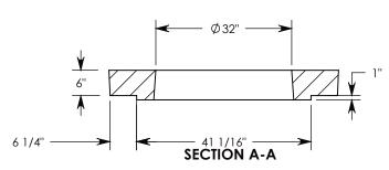
**NOTE 1:** USE OPTIONAL 4" TALL EXTENSION/GRADE RINGS TO INCREASE HEIGHT OF COVER OPENING. P/N: HE-42 **NOTE 2:** CAST IRON MANHOLE LID & FRAME ARE INCLUDED WITH THE FINAL PULL BOX ASSEMBLY.
