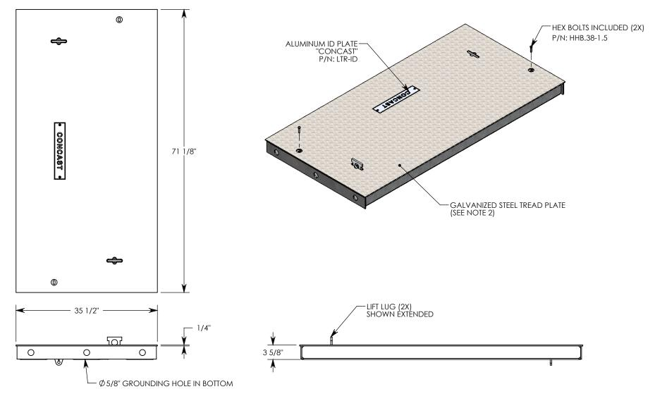
NOTE 1: FOR ADDED SECURITY, PENTA HEAD (P/N: PTA.38-1.5) OR SURELOCK BOLTS (P/N: SL.38-1.25) CAN BE ADDED NOTE 2: TREAD ON DIAMOND PLATE ADDS 1/8" TO OVERALL HEIGHT
