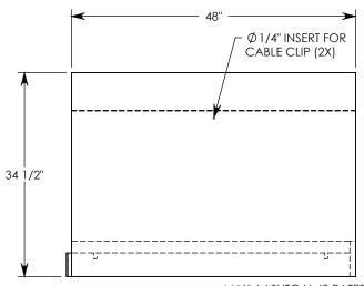
**NOTE 1:** FOR NON-STANDARD LENGTHS THE CHANNEL WILL BE SOLID BOTTOM AND DESIGNATED WITH ITS CORRESPONDING LENGTH MEASUREMENT. IE: 801024HT 32"
