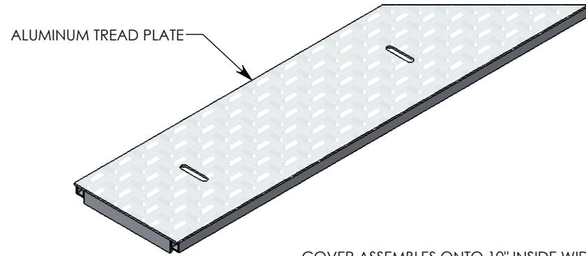
COVER ASSEMBLES ONTO 10" INSIDE WIDTH
