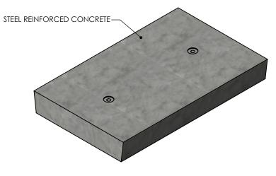
COVER ASSEMBLES ONTO 10" OR 12" INSIDE WIDTH HEAVY TRAFFIC RATED CONCAST HT3 CHANNEL.
