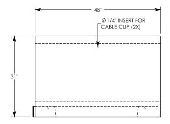
NOTE: FOR NON-STANDARD LENGTHS THE CHANNEL WILL BE SOLID BOTTOM AND DESIGNATED WITH ITS CORRESPONDING LENGTH MEASUREMENT. IE: 802424LT 32"
