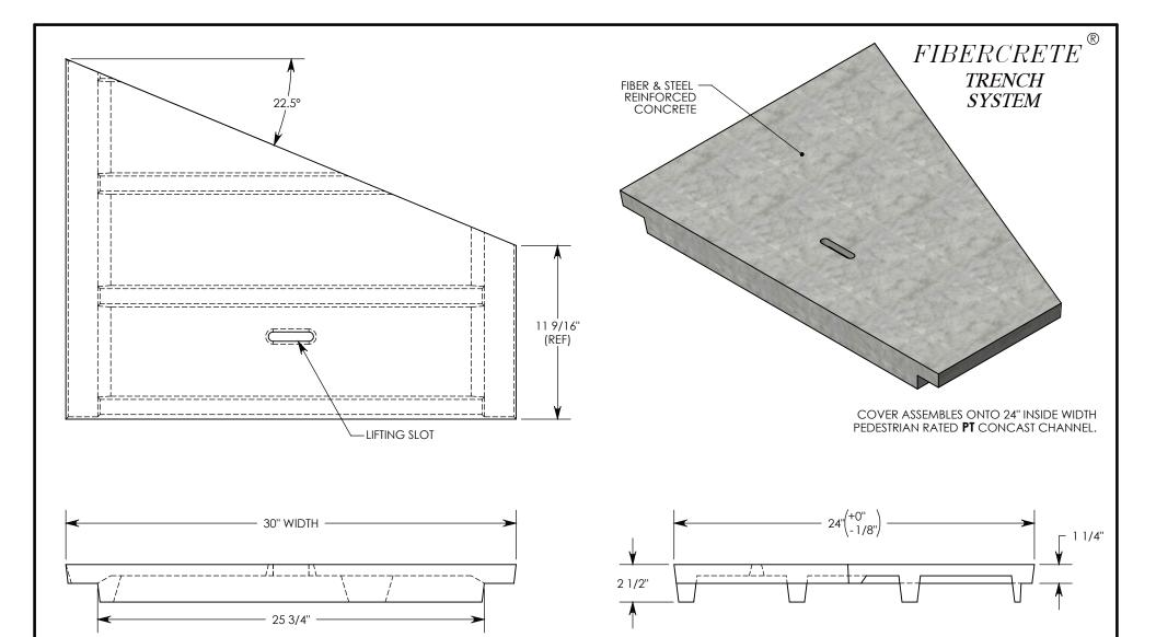
**NOTE 1:** FOR NON-STANDARD LENGTHS, THE PART NUMBER WILL CORRESPOND TO IT'S MEASURED LENGTH. IE: 8025PT 22.5R 18"
