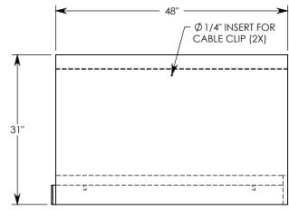
**NOTE 1:** FOR NON-STANDARD LENGTHS THE CHANNEL WILL BE SOLID BOTTOM AND DESIGNATED WITH ITS CORRESPONDING LENGTH MEASUREMENT. IE: 803024HT3 32"
