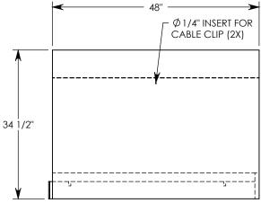
**NOTE 1:** FOR NON-STANDARD LENGTHS THE CHANNEL WILL BE SOLID BOTTOM ANDDESIGNATED WITH ITS CORRESPONDING LENGTH MEASUREMENT. IE: 803024HTSB 32"
