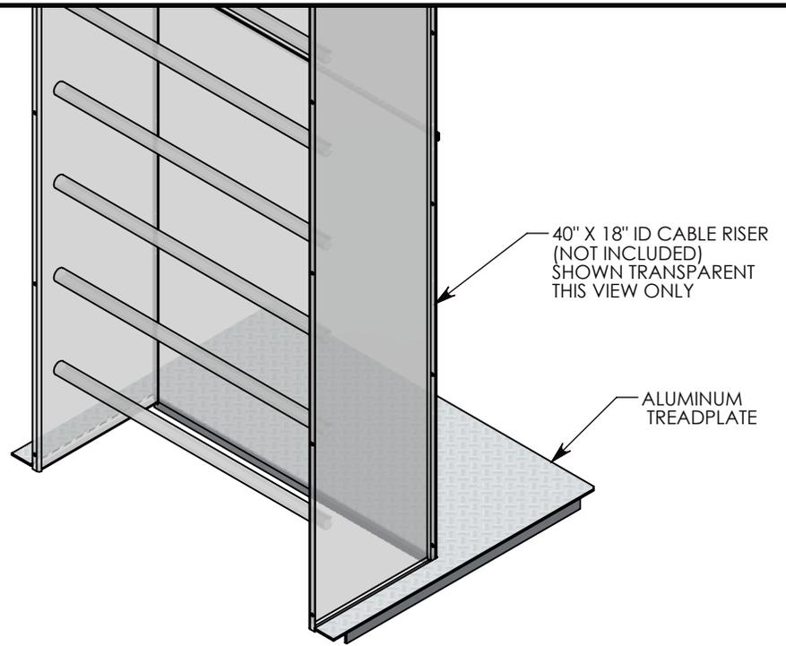
COVER ASSEMBLES ONTO 30" INSIDE WIDTH LIGHT TRAFFIC RATED CONCAST LT CHANNEL.
