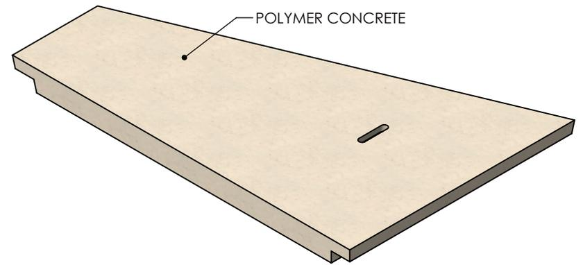
COVER ASSEMBLES ONTO 30" INSIDE WIDTH
