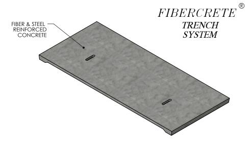
COVER ASSEMBLES ONTO 40" INSIDE WIDTH PEDESTRIAN RATED CONCAST **PT** CHANNEL.
