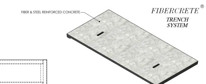
COVER ASSEMBLES ONTO 40" INSIDE WIDTH PEDESTRIAN RATED CONCAST CHANNEL.
