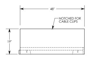
**NOTE:** FOR NON-STANDARD LENGTHS THE CHANNEL WILL BE SOLID BOTTOM AND DESIGNATED WITH ITS CORRESPONDING LENGTH MEASUREMENT. IE: 805016PT 32"
