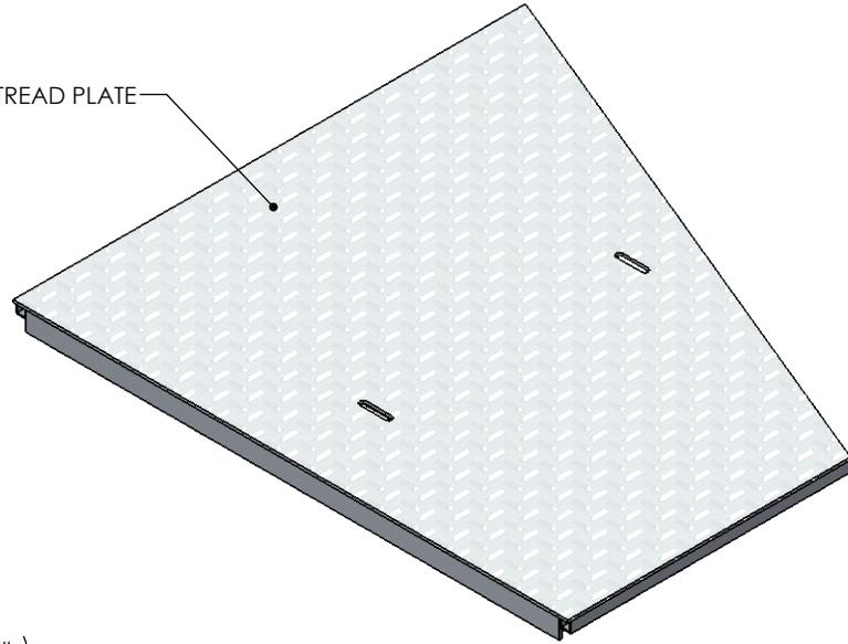
COVER ASSEMBLES ONTO 50" INSIDE WIDTH PEDESTRIAN RATED CONCAST CHANNEL
