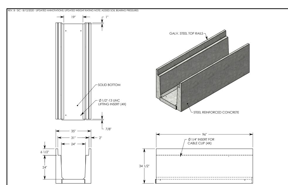
**NOTE 1:** FOR NON-STANDARD LENGTHS THE CHANNEL WILL BE SOLID BOTTOM AND DESIGNATED WITH ITS CORRESPONDING LENGTH MEASUREMENT. IE: 802424HT 32"
